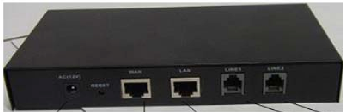
12V/2A adapter Wan Interface Lan interface Ordinary telephone interface
